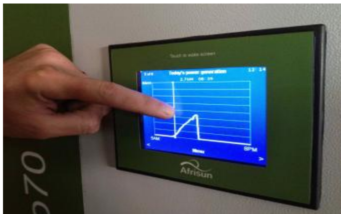
Picture 3: Solar control software for the 70kW grid-tie solar inverter developed by Neil of GreenSparks
