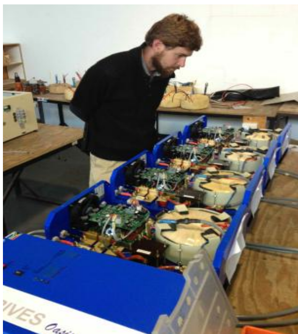
Picture 5: Neil inspecting 4kVA inverters prior to shipping to GreenSparks, Harare
